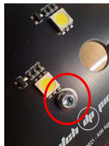
Washer installed, must be removed
